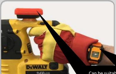
\* Even if a HAV monitor contains an accelerometer, it is not compliant to ISO5349 if the accelerometer is not directly and firmly attached within 10mm of the grip point of a tool.
